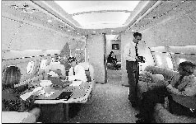
The extra seven-plus inches of the A319CJ's 12.1-foot-wide cabin, compared to the next largest business jet, allows appreciably larger sleeping rooms and private offices while preserving an adequately wide passageway, according to Airbus.
